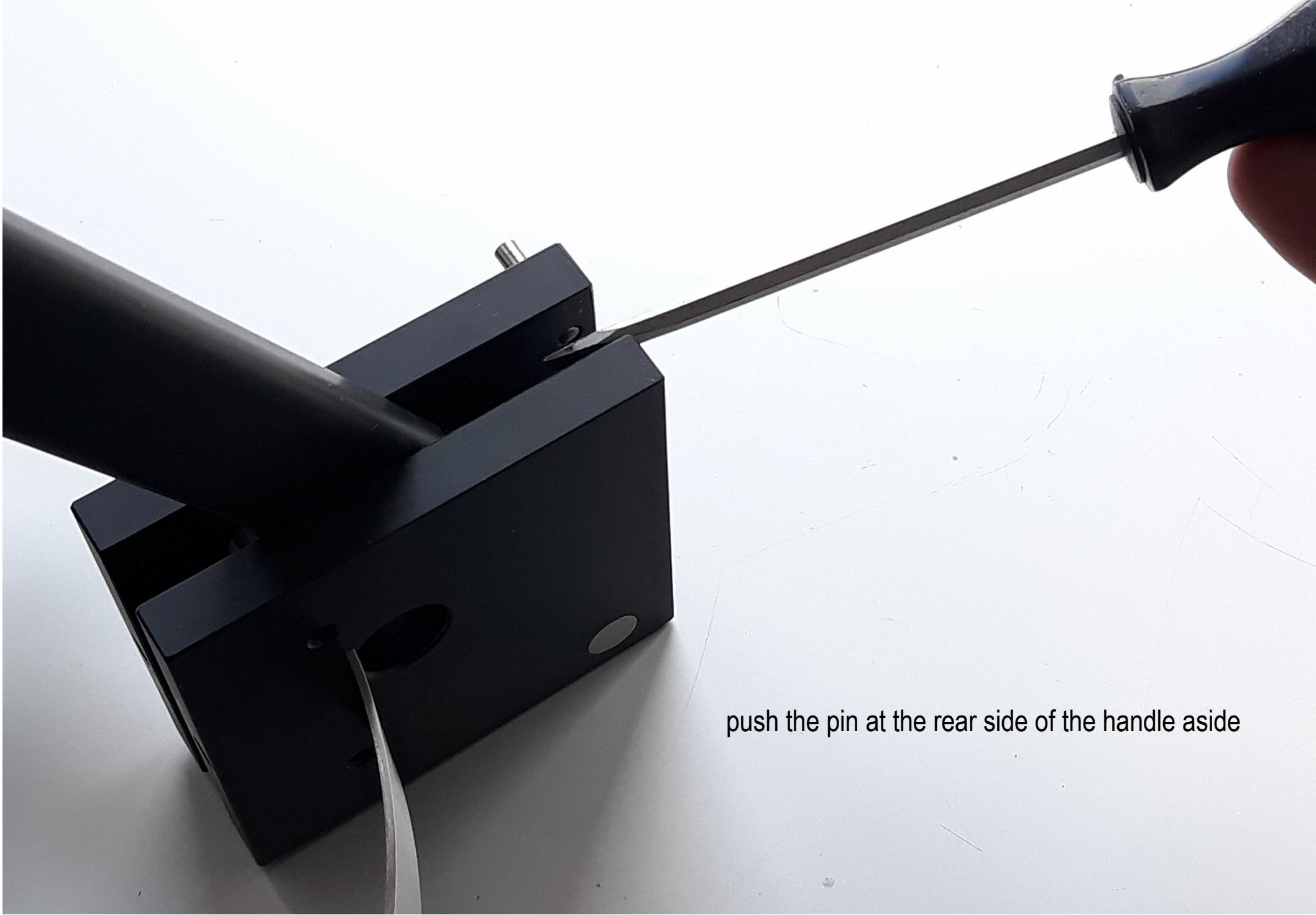
push the pin at the rear side of the handle aside
